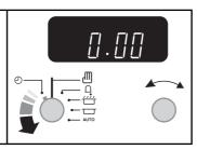
At the same time turn the Adjusting knob left or right until the clock shows the time of day. .
